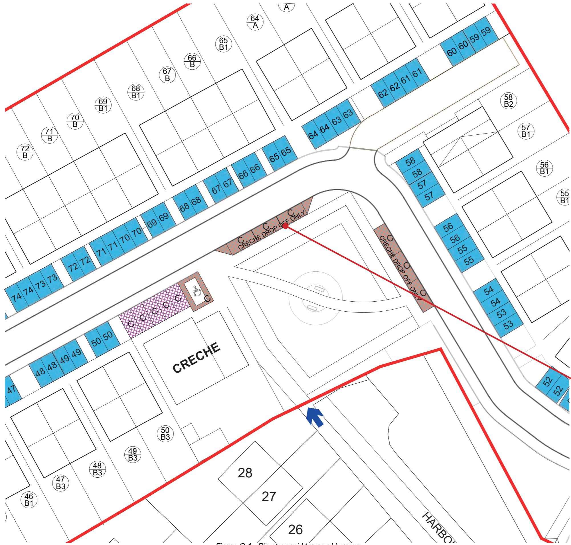
Figure O.1 - Bin store mid terraced houses
